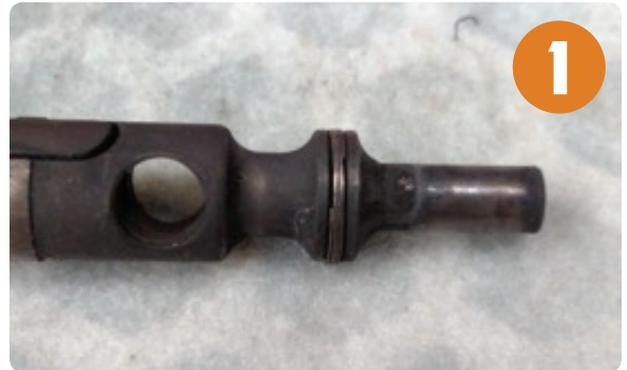
Scrape thick buildup with tool or knife blade.
