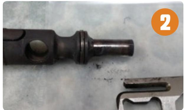
Solvent cleaning with a fabric cloth removes excess fouling (depending on how old the residue is and the original condition of the bolt).
