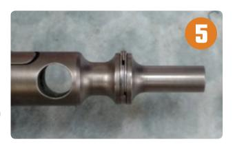
Polish with compound using cloth or Dremel to get the smooth shiny luster back for the ultimate in minimizing fouling adherence.
