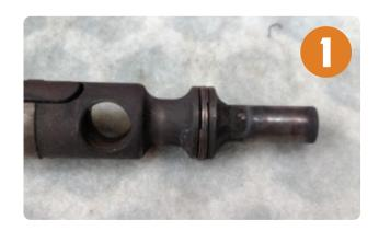
Scrape thick buildup with tool or knife blade.
